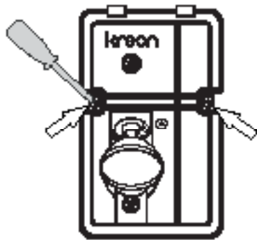
3. Fasten screws until the luminaire is fixed
