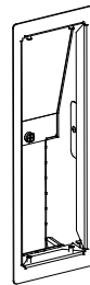
5. Replace the j-box in the luminaire and close the j-box with the cover
