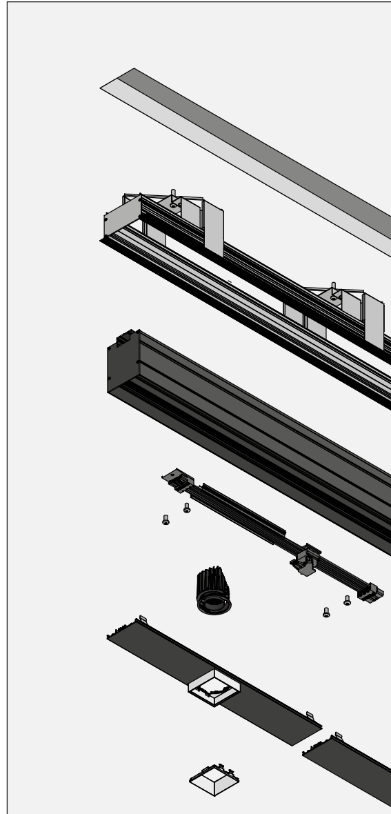
Schematic representation of assembly Prologe 80 single in-Cana: plasterkit + luminaire + louvre
