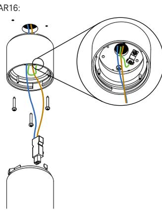
fix the ceilingbox with three screws
