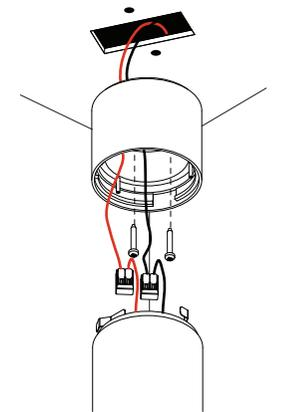
fix the ceilingbox with two screws
