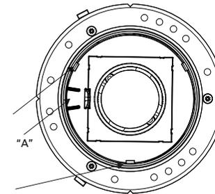
With a round plaster kit, place the ribs "A" between the springs to allow the reflector to rotate for orienting the flower pattern.
