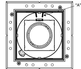
In case of a square plasterkit place ribs "A" "around" the spring for aligning the flower pattern with the sides of the louver.
