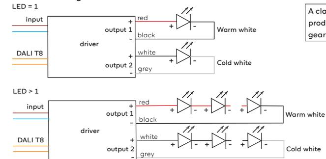
A class III-product or a string of these products in series, can only be used with a gear where  $U_{out} \leq 120VDC!$
