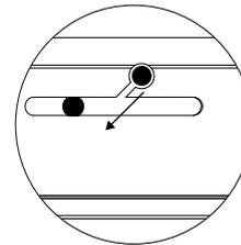
Pull the safety cable all the way to the slot
