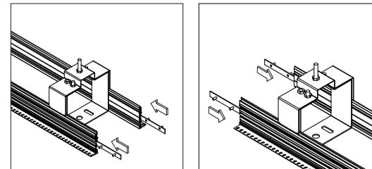
Fix the profiles with the long bracket and the nuts
