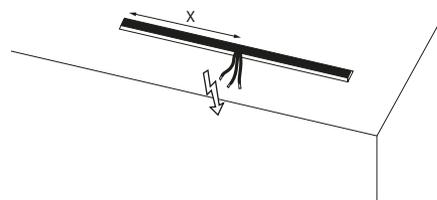
Do not use the profile as or on position of settlement joint.
