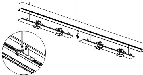
cross connect the modules with each other. each set of connectors has a matching letter (A-A, B-B, etc.) when all the modules are connected, connect the modules to the driver with the provided connector
