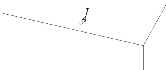
install the top part of the gearbox and wire grip. plugs and screws are not supplied, choose correct plugs and screws according to the material of the ceiling surface
