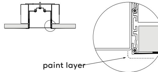
Don't remove the aluminium brackets, screws need to be reused for mounting the main profile
