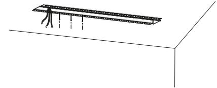
Use included high performance gypsum screws for fixing flange. Distance between screws 100-200mm.
