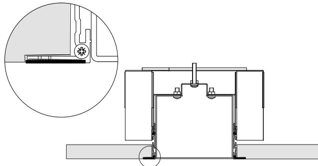
add 3mm of paint on the inside of the profile. This area may be visible after installing the main profile
