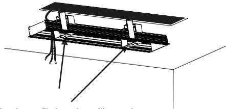
Put the profile into the ceiling and don't remove sheet metal brackets.
