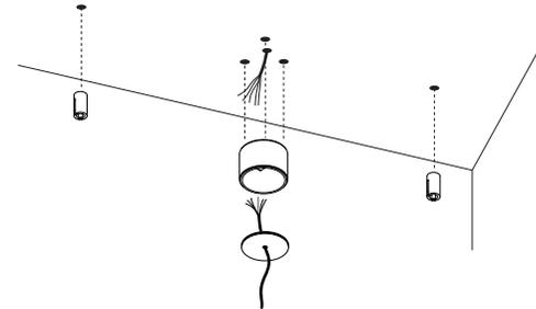
fix steel cables to wire grippers and adjust to the correct height. Connect power supply to luminaire
