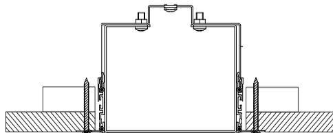
Add Gypsum fleece band (preferred) and fill around perimeter of plasterkit using suitable fiber-reinforced filler and plaster to hide screws and plasterkit.
