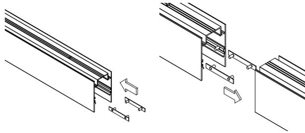
Fix the profiles with the long bracket and the nuts
