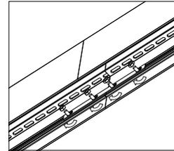
arrange the modules on a clean table before installing. Modules are labeled 1 2, 3 4, 5 6...7 8. Nr. 1 inside profile indicates where to start
