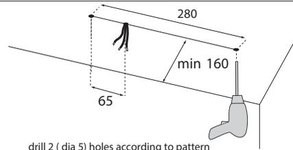
drill 2 ( dia 5) holes according to pattern
