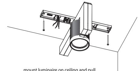
mount luminaire on ceiling and pull
