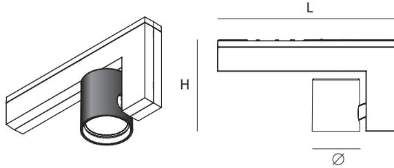
remark: due to the high temperature that occurs on the adjustable part, the luminaire must be placed out of arms reach
