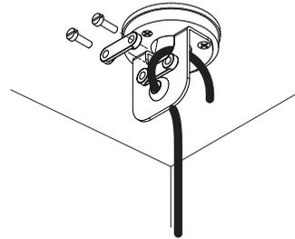
Loop cable through top hole and fixate cable
