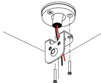
Add the cable bracket to the installation part by fixing it with two screws
