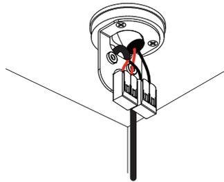
Connect cables by using connectors
