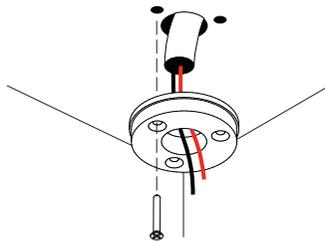
Pull the cable through the center hole and fix installation part to the ceiling with 1 screw
