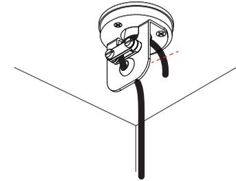
Cut the cable after the loop
