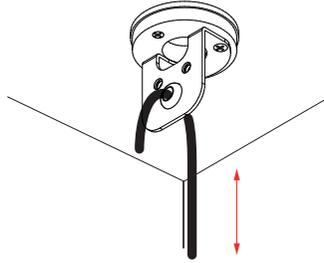
Feed suspension cable through the grommet
