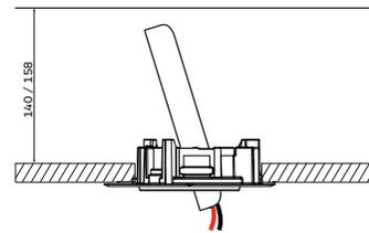
In case of other gear, length gear + 30mm
