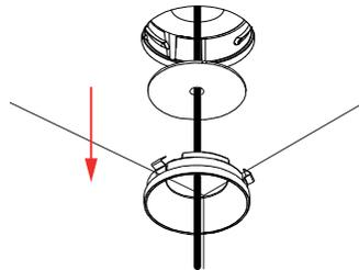
Insert tool in the locking system with the correct way up
