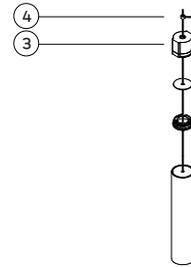
Tighten cable gland at the desired suspension height using the included tool
