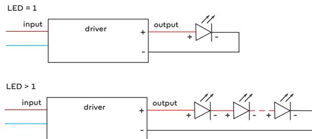
A class III-product or a string of these products in series, can only be used with a gear where  $U_{out} \leq 120VDC!$
