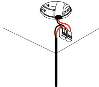
Align plasterlock with plasterkit and insert locking mechanism using the tool
