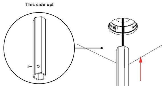
Insert hex key in the small hole of the plaster lock
