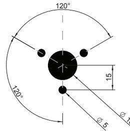
Drill three holes of  $\varnothing 5\text{mm}$  (depth min. 40mm) for the plugs and drill one hole in the middle of  $\pm \varnothing 18\text{mm}$  for the cable
