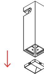
Remove the housing by sliding it down
