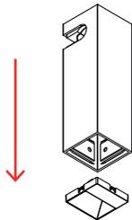
Open the sliders by turning the screw, using the included tool
