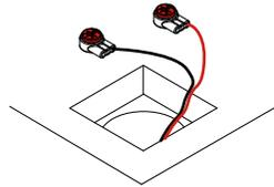
place the wires coming from the up fixture on the side of the connectors: match red with red and black with black
