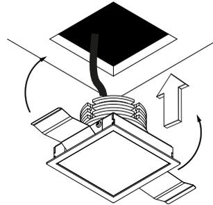
fold the springs against the fixture and rotate
