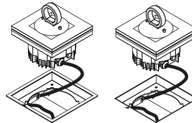
when installed in a hollow floor (no matchbox)
