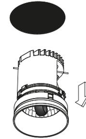
Pull the complete fixture out of the ceiling
