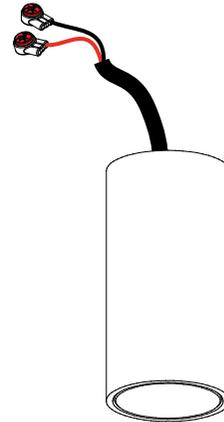
place the wires coming from the up fixture in the delivered connectors (or any desired connector with the correct IP-rate) :
