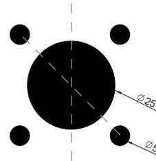
Drill four holes of  $\varnothing 5\text{mm}$  (depth min. 40mm) for the plugs and drill one hole in the middle of  $\pm \varnothing 25\text{mm}$  for the cable
