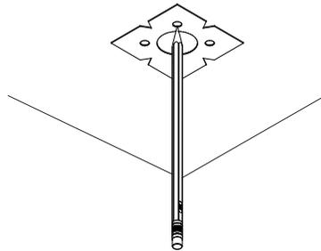
The delivered mold can be used to indicate the fixation holes on the ceiling
