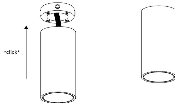
Click the up fixture over the installation part on the ceiling. All four springs need to click
