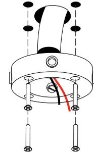
Pull the cable through the center hole and fix installation part to the ceiling with 4 screws
