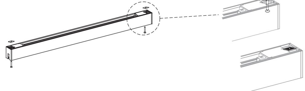
set the nut on top of the screw
