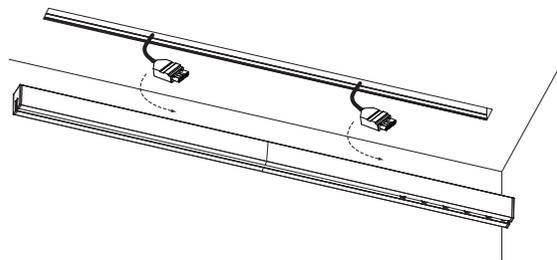
fix the luminaire in the installed recessed profile
