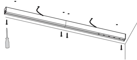
cover screw holes with supplied tube plugs
