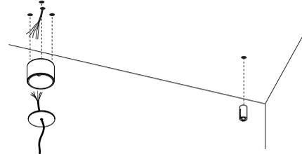
fix steel cables to wire grippers and adjust to the correct height
