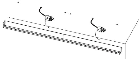
fix the luminaire to the ceiling with screws
