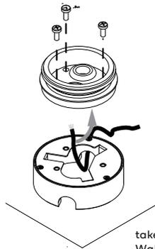
take the installation part that is delivered with the Wabi fixture itself and mount it with the 3x M5 screws onto the spacer. Pull the cable through the holes of the installation part
