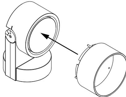
make sure to align the screws in the glare preventor with the threads in the head of Wabi
