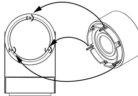
fix the three screws with the included hex key
