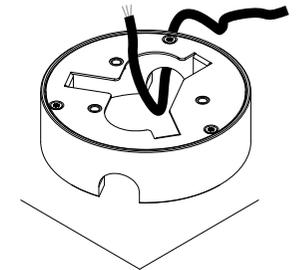
drill mounting holes in the indicated position
