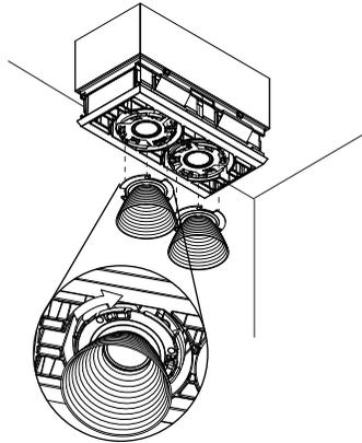
when installing the reflectors again, slide the bumps on the reflector under the cavities in the reflector holder
