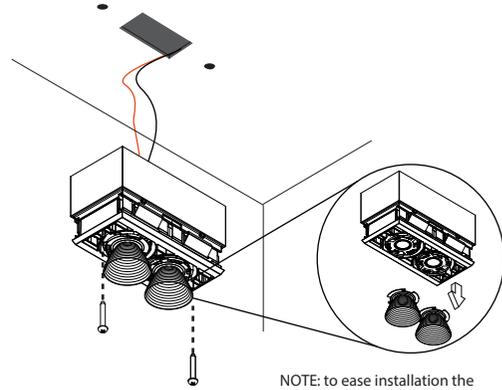
NOTE: to ease installation the reflectors can easily be taken out by rotating counter clockwise and then pulling down
