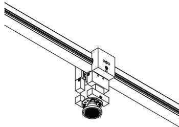
Close the sliders using the tool, make sure no cables are pinched
