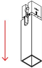
Open the sliders by turning the screw, using the tool from KR754911, or a hex key, until you feel the blocking mechanism
