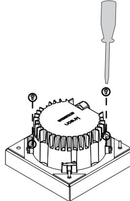
fix the brackets with the two delivered screws
