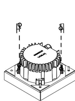
align the flanges of the two delivered brackets with the cavities in the free details at the back of the product
