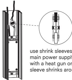
use shrink sleeves to make connection with main power supply, heat the shrink sleeve with a heat gun or lighter until the sleeve shrinks around the cable.
